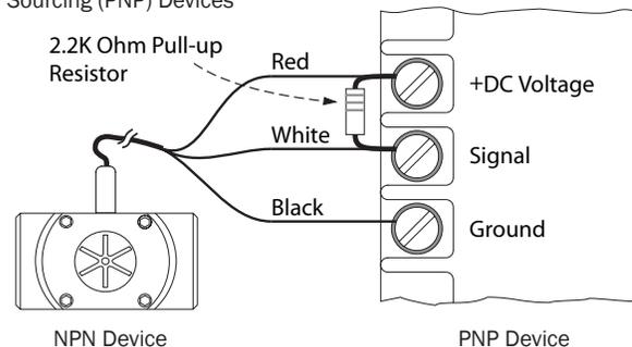
Since the three-wire pickup sensors are solid state, they do not exhibit switch bounce and can be used at relatively high frequencies.
