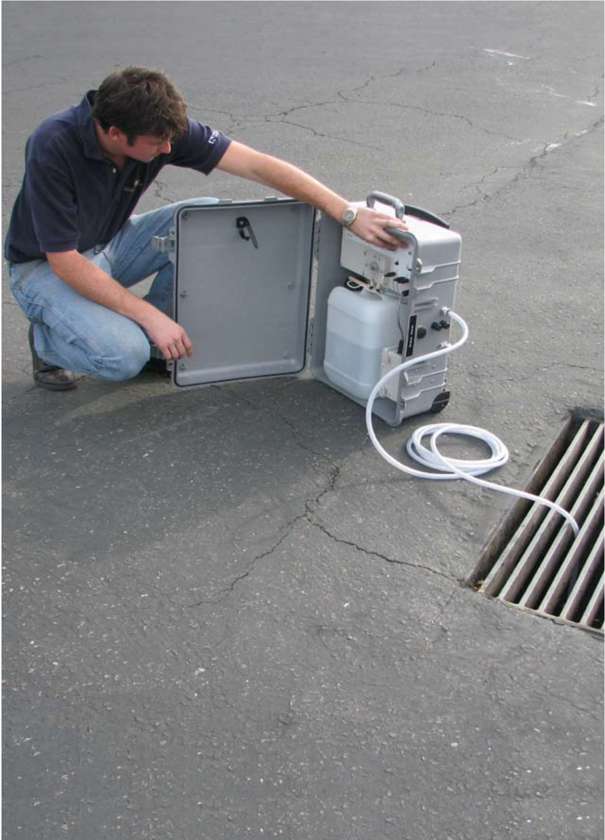
Monitoring stormwater drainage with a Global Water WS705 water sampler.
